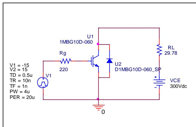
Test condition:  $I_C=10$  (A),  $V_{CC}=300$  (V)
