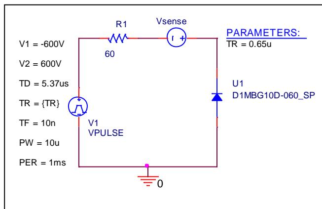
Test condition: VCC=600 (V), IC=10 (A),  $-di/dt=30A/\mu sec$
